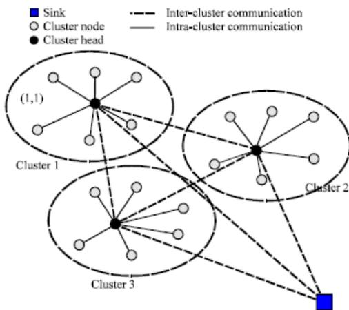
Fig. 1. Architecture of Clustering in WSN
